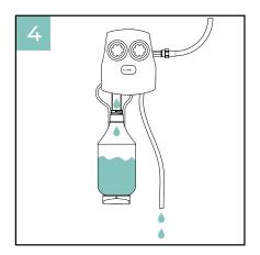
When the solution is activated the unit will beep and the blue light returns to green. The solution is now ready to dispense. The dispensers are set to deliver 20L at 100ppm via the bottle dispenser and 30L at 50ppm via the hose dispenser. The water pressure needs to be between 2 to 5 bar for the correct ppm to be made.
