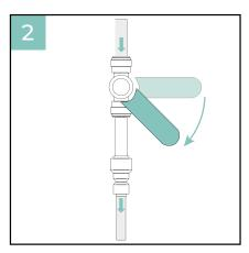
Open the lever valve to fill the tank up to the 5L mark.
