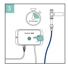
Switch on the activator unit - the unit's light button will turn green. To activate press the green light button. It will turn blue and the activation process starts, which takes 45 minutes. You will see bubbles around the cell and a faint smell of chlorine once activated.
