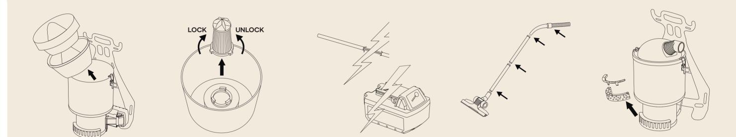
Replace the paper or SMS disposable dust bag if needed. Remove, empty and clean the reusable dust baa.
